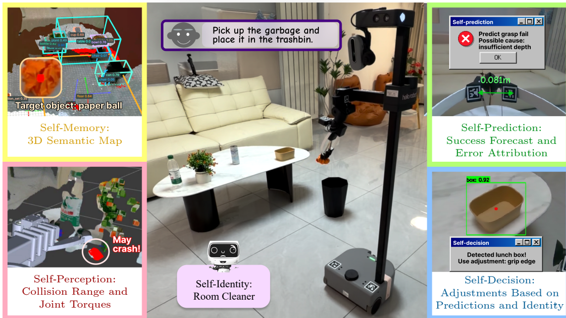
Fig.6. Overview of real-world experiments on the Stretch robot. The proposed self model is evaluated in real environments through its four components, including self-perception, self-memory, self-prediction, and self-decision. These components support embodied tasks such as navigation and manipulation, enabling the agent to perform them more effectively.
